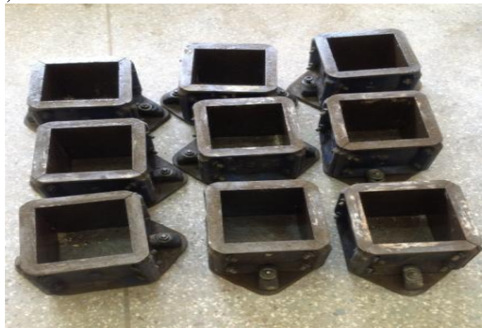
Fig 1 Cast iron moulds
